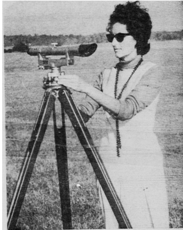
FIRST CIVILIAN WOMAN surveyor in the Air Force, Mrs. Audrey McGlothlin adjusts the balance of her surveyor's level before taking an elevation reading. Mrs. McGlothlin completed the Site Development Specialist School, Sheppard AFB, Tex., with the third highest rating in her class. She is assigned to the 3380th Civil Engineering Group here. (U. S. Air Force Photo by SSgt. George Hill)
